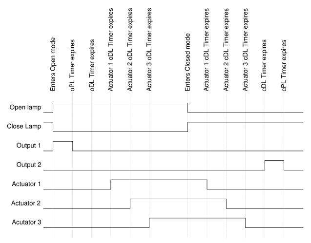
Figure 6 - Conveying System Timing Diagram
